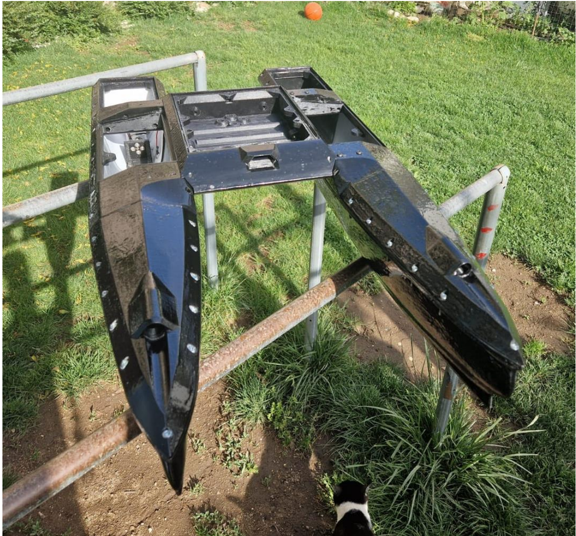
Figure 5.3: The fully assembled vehicle structure prior to electronics integration, highlighting the mechanical M5 bolt connections and plexiglass viewports.
