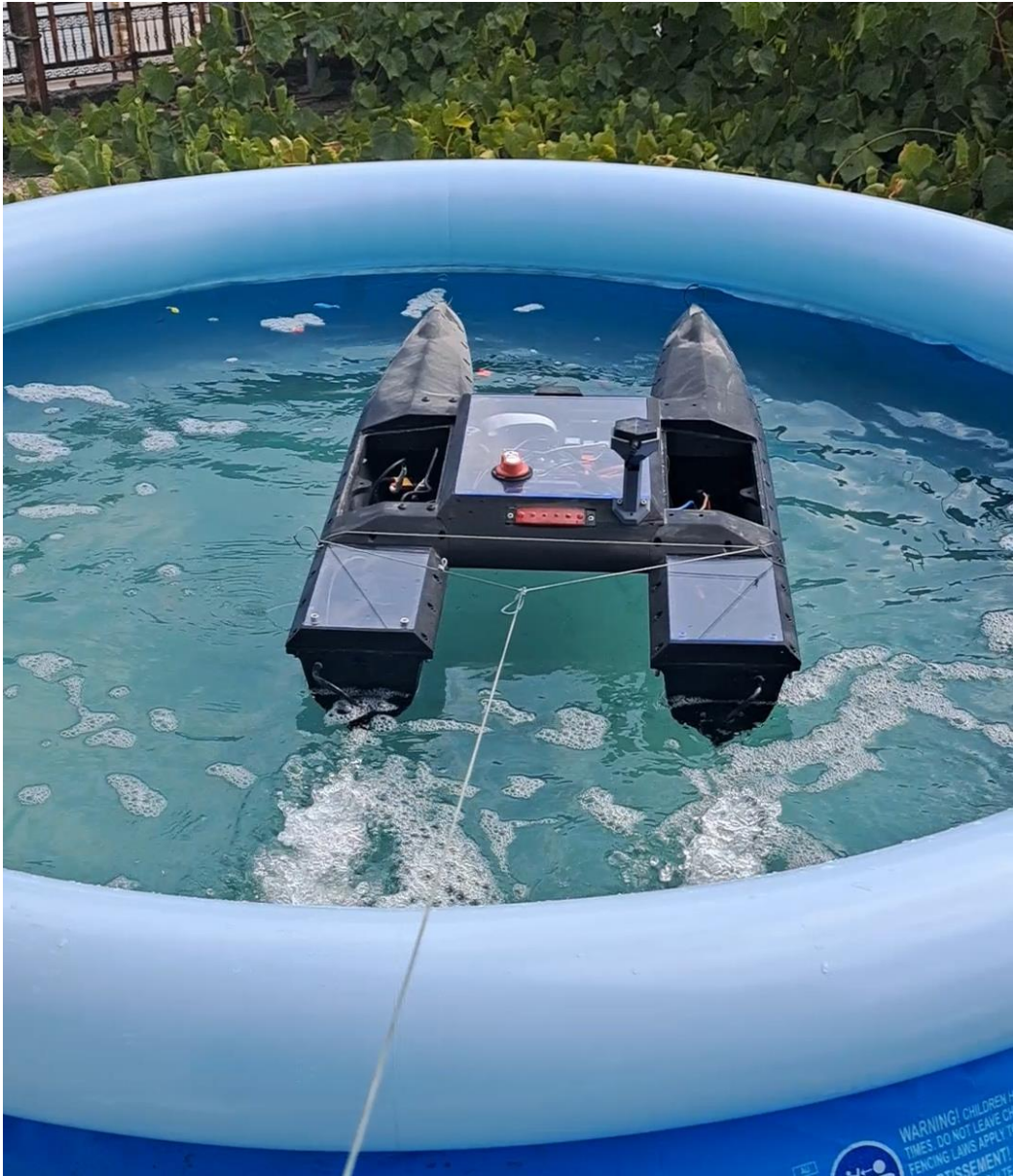
Figure 5.6: Initial buoyancy and watertight integrity test conducted under controlled conditions. The ASV is shown floating under full operational mass during low-speed propulsion activation, demonstrating stable flotation and absence of immediate water ingress.
