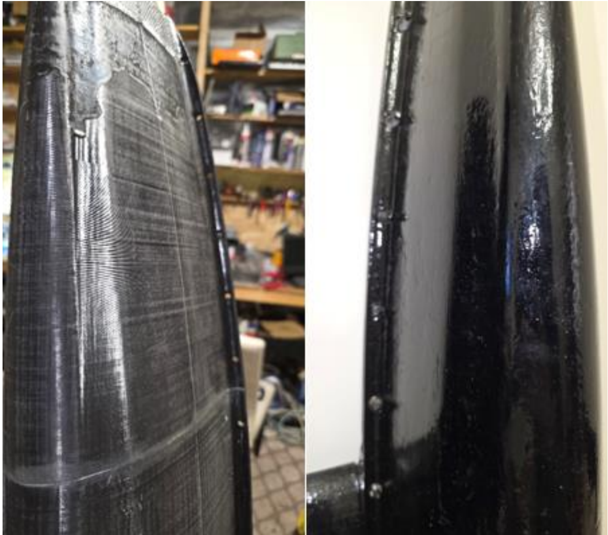
Figure 5.2: The hull sections before and after undergoing the epoxy coating process. The glossy finish indicates the sealed surface preventing water ingress.
