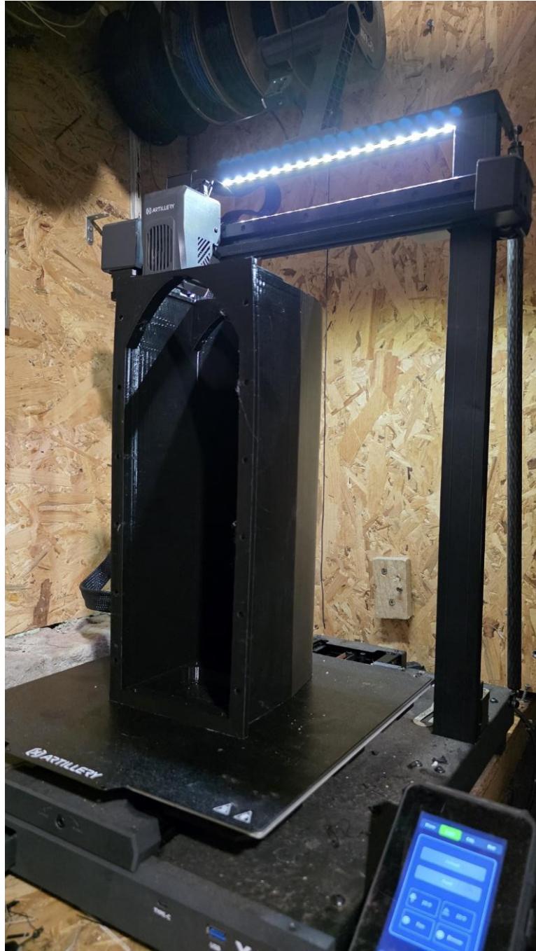
Figure 5.1: Fabrication of hull segments with 3D printer.
