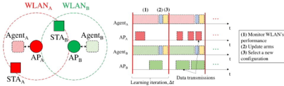
Figure 2. 14 A scenario of two overlapping WLANs and the agents learning procedure [18]
