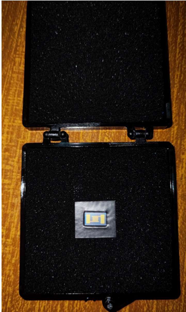
Figure 5.16: Real life dimensions and picture of the interdigitated electrode that will be used as a sensor for the bacterial capacitance measurement
