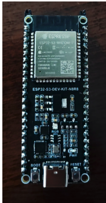
Figure 6.4: The microcontroller ESP32-S3-DEV-KIT-WROOM-1-N8R8 that will be programmed for the proper operation of the circuit
