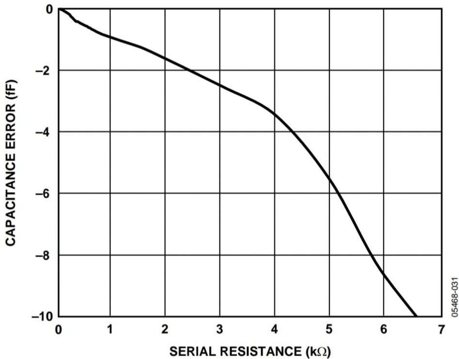
Appendix Figure B.10: Capacitance Input Error vs. Serial Resistance, CIN(+) to EXC = 21 pF, CIN(-) to EXC = 23 pF, VDD = 5 V [19]
