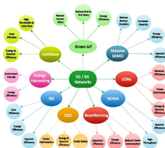
Figure49 Overview of key 5G/6G green communication technologies and their relationship with sustainability indicators [24]
