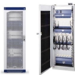
Σχήμα 18: Base Station Controller
