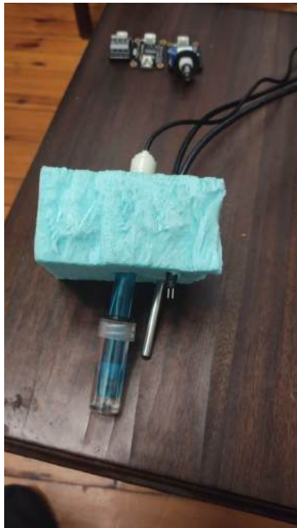
Image 13.8: PH connector setted up at a block of styrofoam in order to float inside the container
