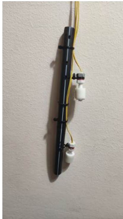
Image 13.9: Construction of the two float sensors that will go inside the container
