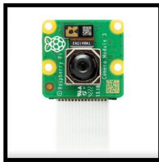
Σχήμα 5.3: Raspberry Pi Camera Module V3 - Standard 11.9MP 75° [7]
