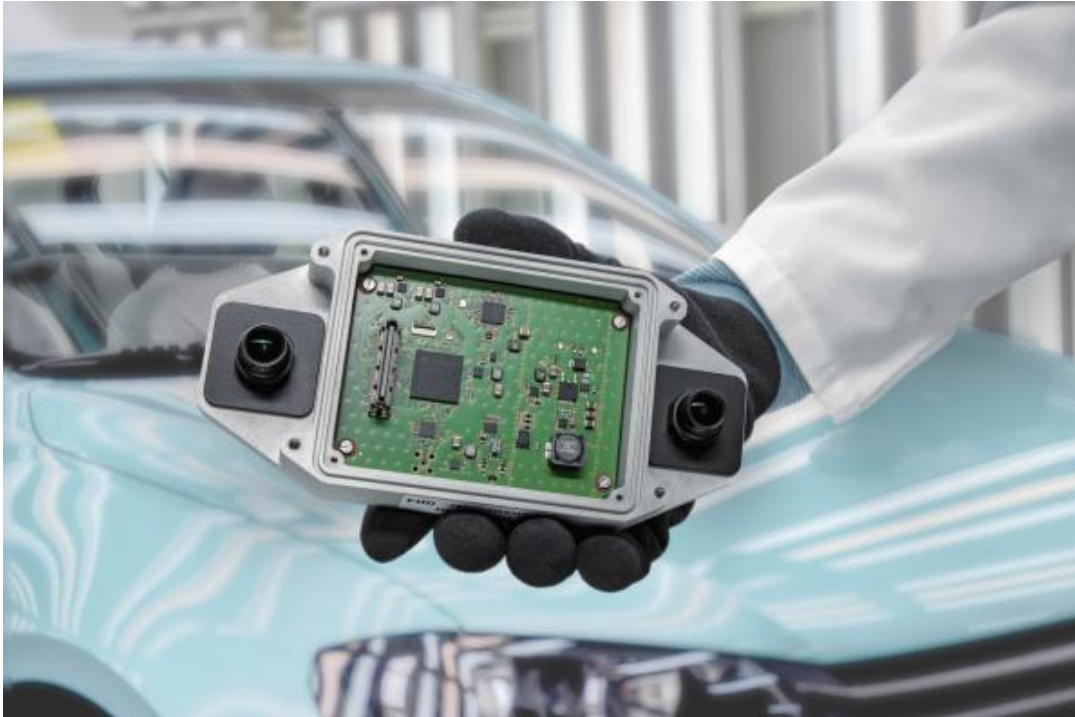
Figure 2.5: A radar alongside a camera module. [19]
