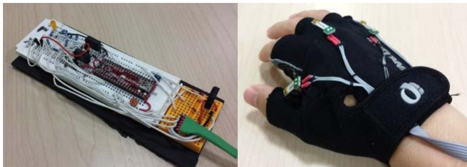
Figure 3 Tactile Teacher Prototype with a microcontroller (left) directly connected to an instrumented glove (right) [24]
