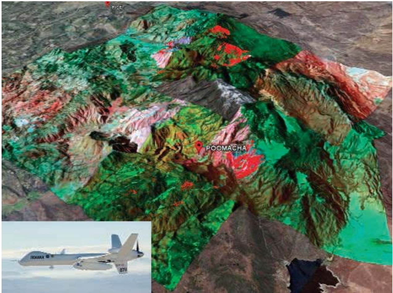
Figure 19 Thermal-infrared images from the unmanned Ikhana (inset) helped firefighters battle the Poomacha fire near San Diego’s Palomar Observatory [44].
