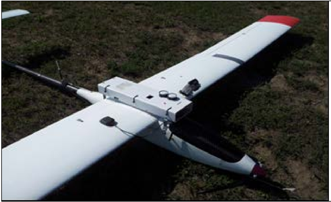
Figure 15 Fix wing drone equipped with chemical sensors [21]
