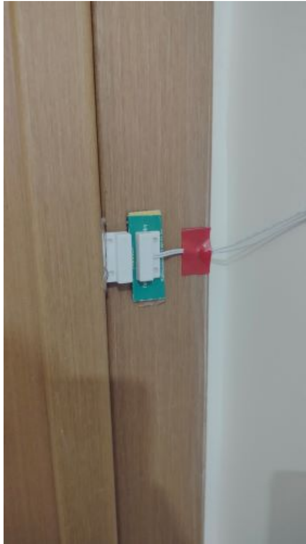
Figure 4.13: The magnetic lock sensors are placed on the door and door frame
