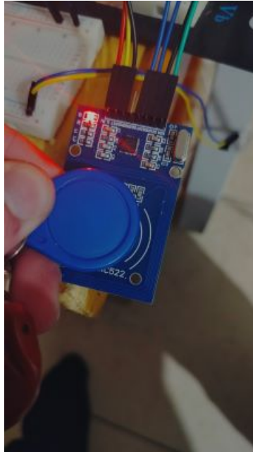
Figure 4.12: Using an authorized RFID tag we gain access to the house
