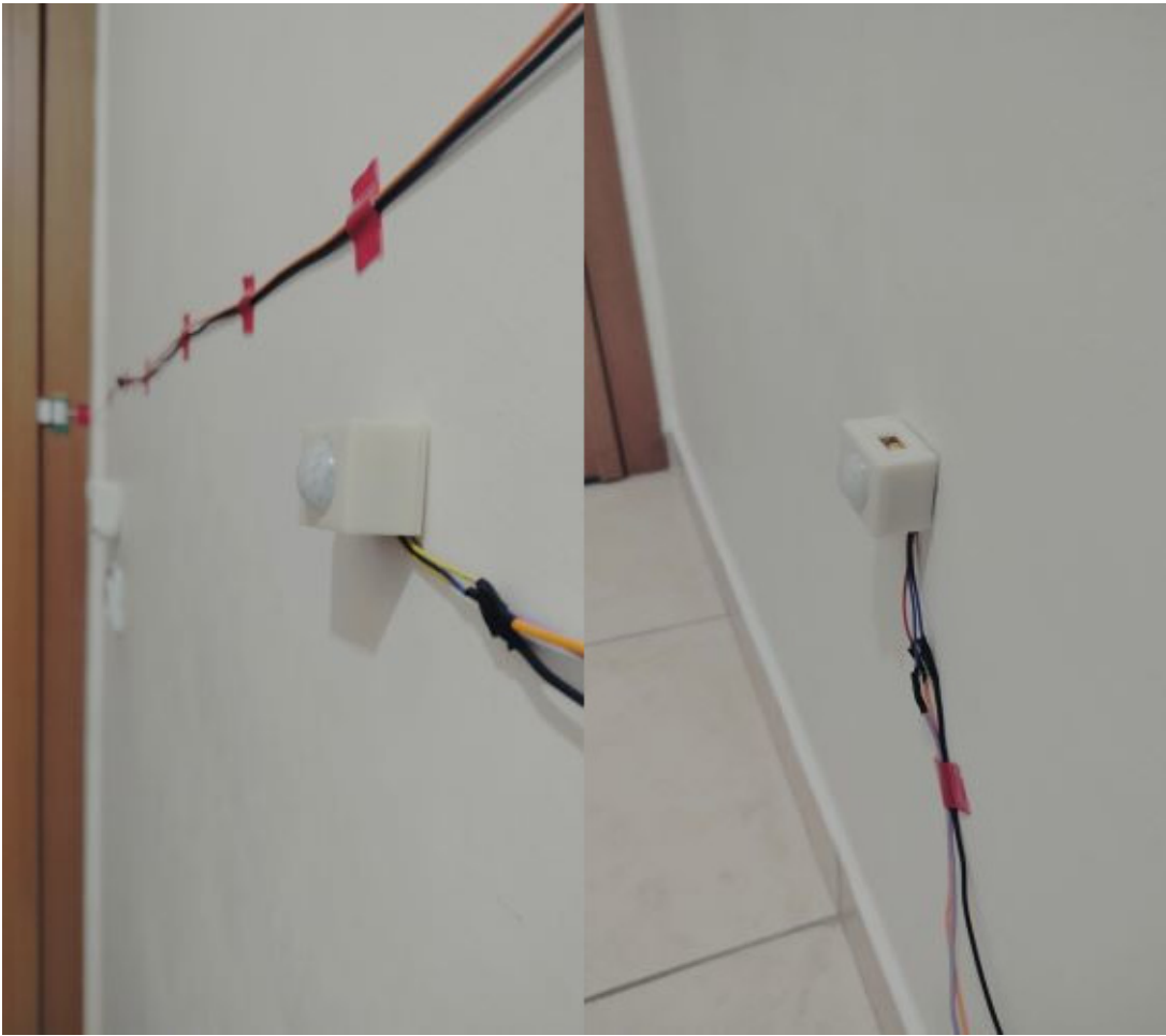
Figure 4.14: Using the PIR sensors we can detect who is passing though (left for humans, right for pets)
