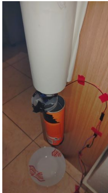
Figure 4.8: The servo motor is placed in the opening of the container. When we press the button, the servo will rotate the disk, and the food will drop into the small hole
