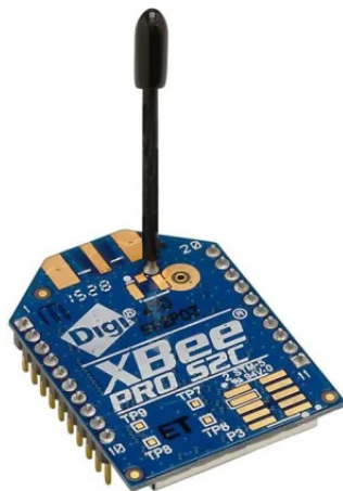
Figure 1.3: The Zigbee module was one of the first wireless- low power technologies for personal area networks
