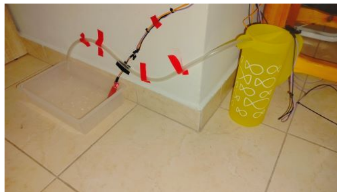
Figure 4.9: Inside the yellow reservoir, the water pump will flow water through the tubes if the water is low thanks to the water level module
