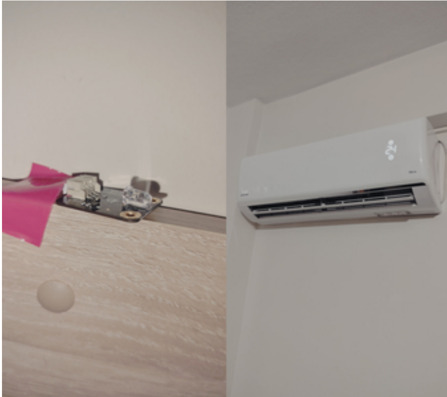
Figure 4.4: Using the IR transmitter module (left) we can control the A/C (right)
