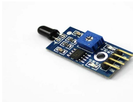
Figure 2.26: Fire Module Source
