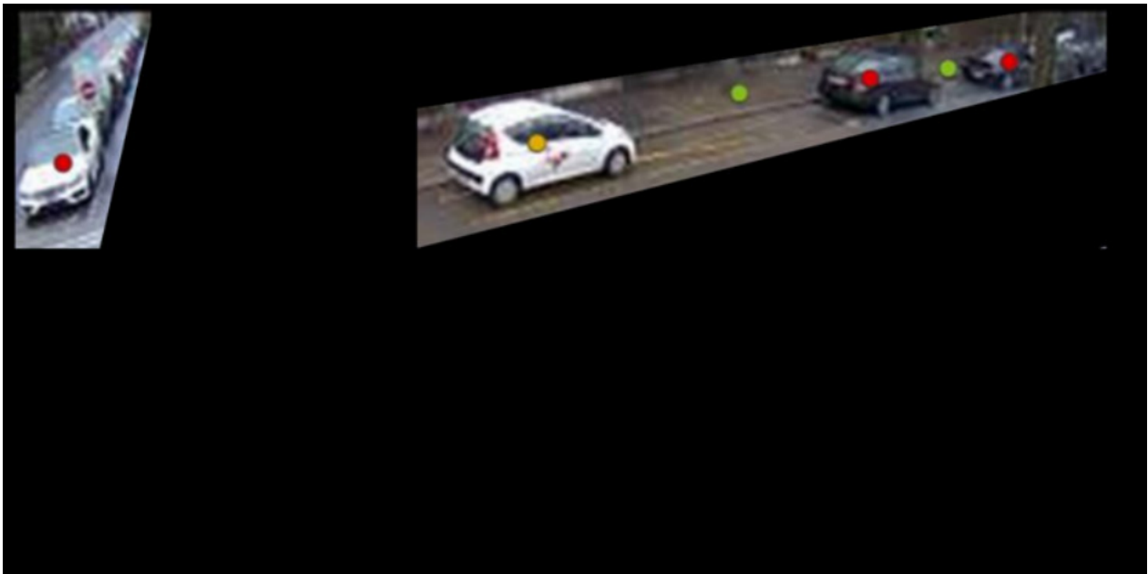
Figure 4.14: Sample output from the privacy-aware low-resolution camera used in the project. Despite limited fidelity, parking occupancy detection remained effective while protecting individual identities. The entire field of view, except for the parking spots, is blacked out to ensure no surrounding personal or identifiable information is visible [111].
