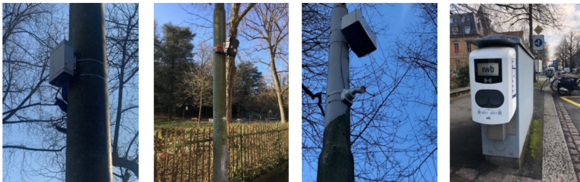
Figure 4.1: Overview of the sensors used in the Basel Smart Road project [111]: from left to right, an air quality sensor, a noise sensor, a traffic monitoring camera, and an electric vehicle charging station.
