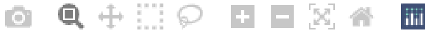
Figure 3.2: The interactive Plotly toolbar offers users various controls for refining their chart views and interactions [105]. From left to right, these icons enable features such as screenshot capture, zooming, panning, selecting data points (using a box or lasso), autoscaling, resetting the chart view, and toggling specific chart modes.
