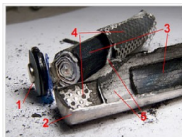
Disassembled NiMH AA battery:
