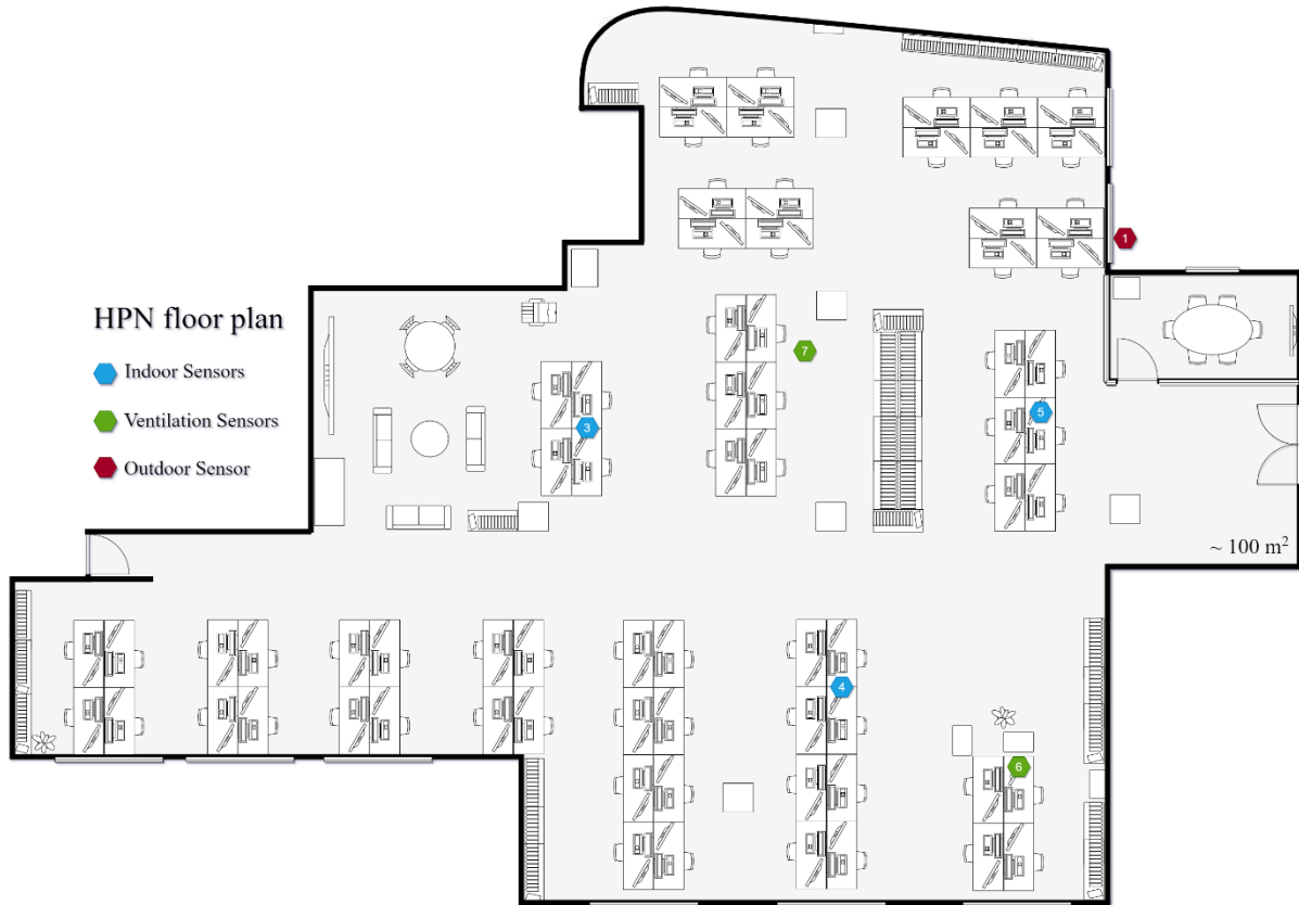
Figure 3.3: Sensor deployment floor plan
